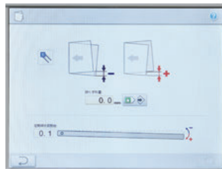
Fine-adjustment for skewed folds sets automatically by entering the skewed fold measurement or shift amount of the sheet register guide.
